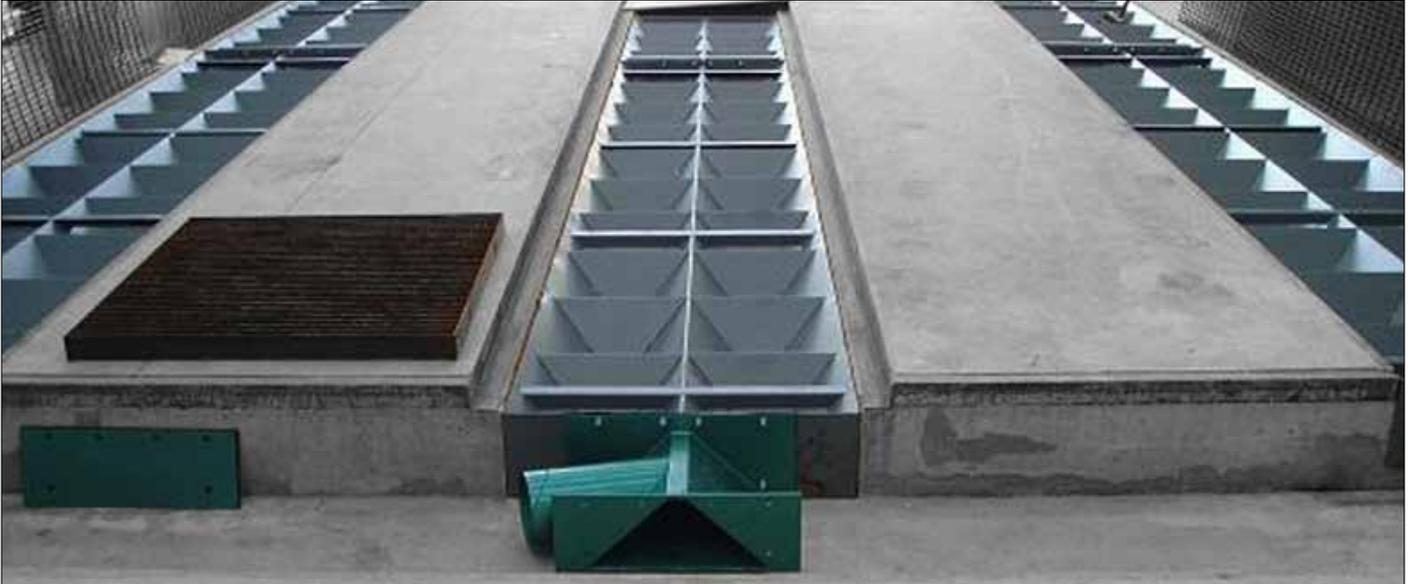
Pictured Above - Three (3) Module ABSS Recovery Floor fitted flush to the Blast Room Floor. Shallow Pits of 280mm are required.
